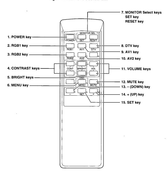
Fig. 1 Wireless remote control unit
